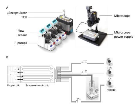
Figure 2  $\mu$ Encapsulator system set up. (A) Image of the system set up depicting all the components of a  $\mu$ Encapsulator. (B) The schematic of the individual fluidic lines driving cells, hydrogel, and oil.
