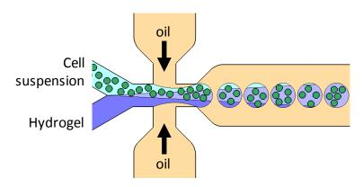
Figure 1 Schematic of hydrogel droplet generation. Tens of thousands of single cells are encapsulated with hydrogel inside droplets.
