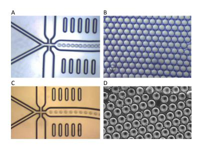
Figure 3 (A) Matrigel and (C) agarose emulsions were produced at the optimal flow rates, and droplet formation imaged at the chip junction.(B) Matrigel and (D) agarose emulsions imaged after formation show high monodispersity.
