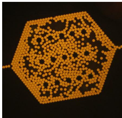
Figure 2: Production of aqueous droplets labelled with Rhodamine G6 (100mM) by using FluoSurf 4 w/w-% in HFE 7500.
