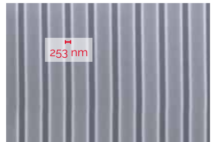
Minimum feature size: 300 nm - or even less. The image shows the result of a high-resolution test exposure with a nominal linewidth of 250 nm!
